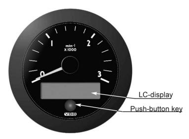
The VDO Ocean Link tachometer is a multifunctional instrument for indicating engine data, and is intended for use in navigation of sports ships. The tachometer shows the actual engine speed in operation, on the analogue scale. Further values and operating aids appear in the LC-display.
