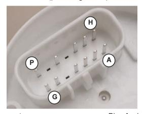
Pin: Assignment: Pin: Assignment: Slave Bus Power Slave Bus Data Н Α В Analogue input 4-20 mA J CAN high Analogue input 0-200 Ohm C K CAN low Slave Bus Ground / Signal Ground D L Vacant Ε M Cl. 58 (illumination) Vacant F CI. 31 (GND) N Vacant G Cl. 30 (continuous voltage) Р Cl. 15 (ignition)
